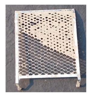
Painting grate during clean-up (DSCN0864.jpeg). Each grate has about 360 holes, which can be cleaned at the rate of about 7 seconds per hole.
