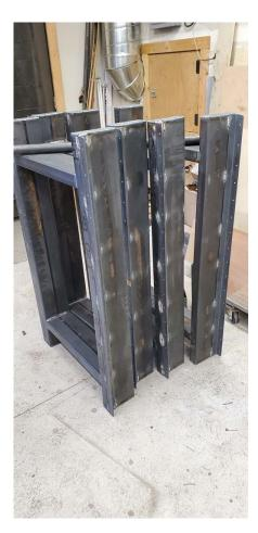
Left: Welded frames for carriage-mounted benches.
